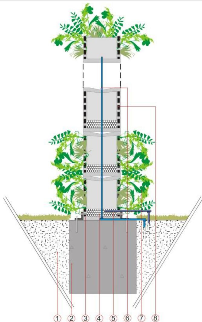
Side view of system-bound facade greening (here with the addition of a foundation)
