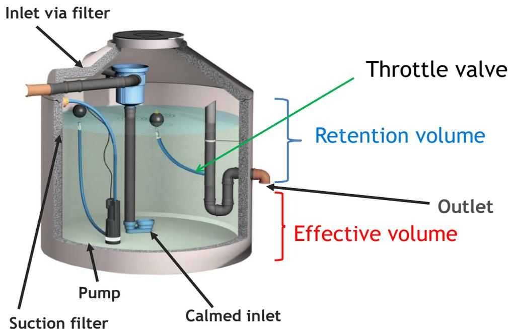
A conflict exists between rainwater utilisation (cistern should be full at all times) and the hydraulic relief of sewer (cistern should preferably be always empty, in order to collect new runoff). Retention cisterns are constructed as a combination structure to fulfill both demands. They have a specific **retention volume**, which can be throttled discharged into sewer and an additional fixed **effective volume** for reuse.
