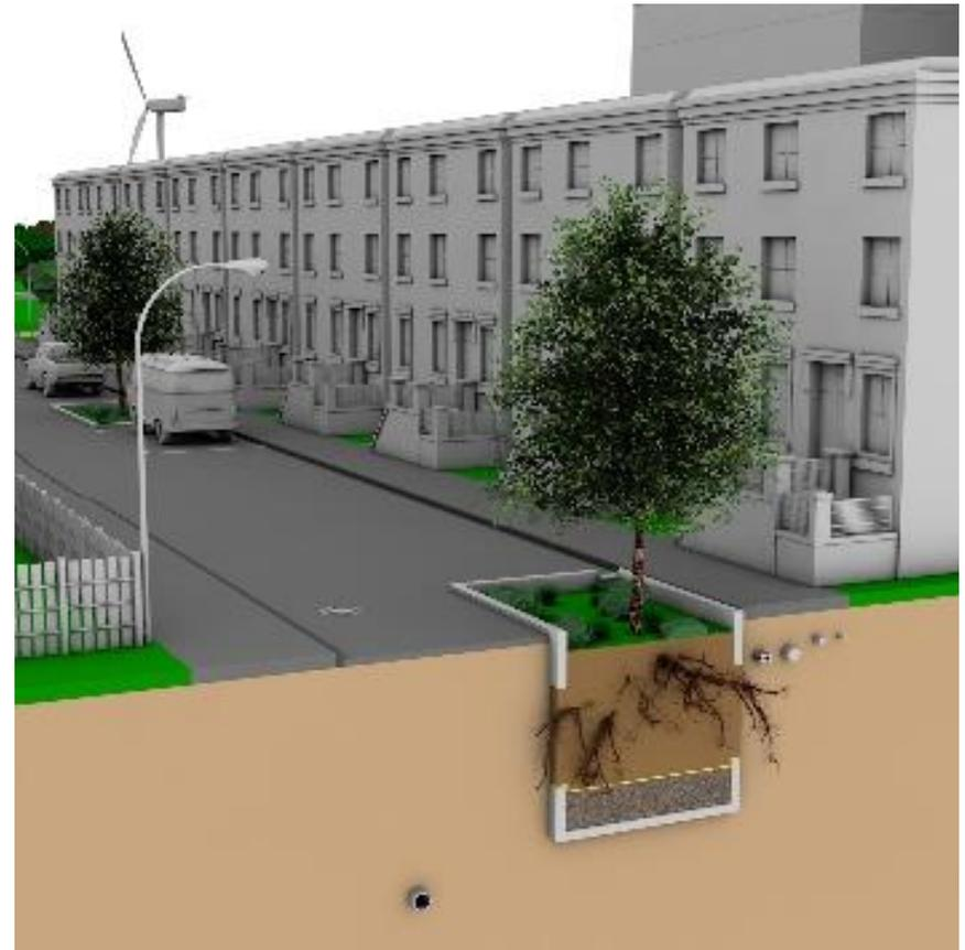
Schematic diagram of a tree-trench system (tree box) (Source: Sieker)
