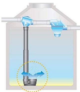
A calmed inlet prevents whirl up of sediment at the bottom of the rainwater tank
