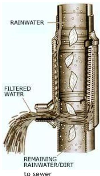
A downpipe filter collector diverts 90% of the rainwater to a storage tank through a 0.17 mm stainless steel mesh filter
