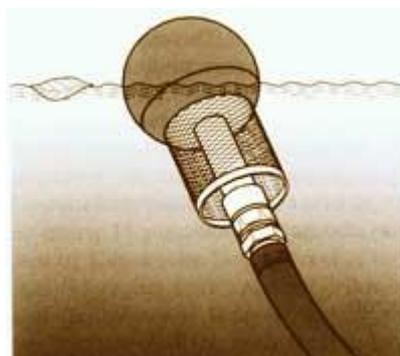
A floating fine suction filter ensures that rainwater is pumped from cleanest level of the tank and is free of particulates
