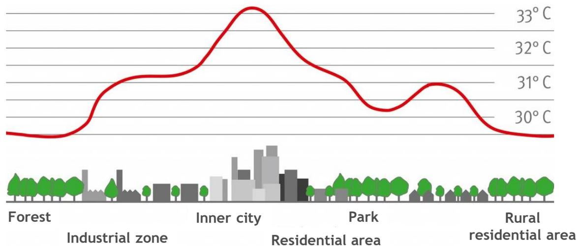
Increased sealing of surfaces, less green and rapid discharge of rainwater away from city will increase the heat island effects
