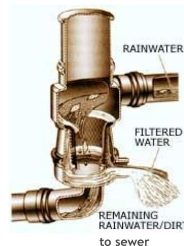
A large vortex fine filter diverts 90% of rainwater runoff from roof areas of up to 500 m<sup>2</sup>
