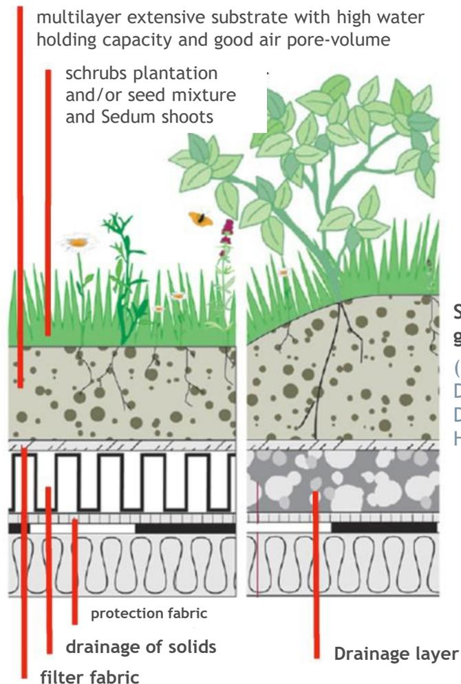
Setup of an extensive green roof
