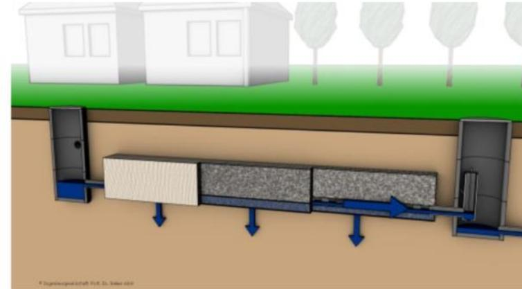
Schematic diagram of an infiltration trench with
