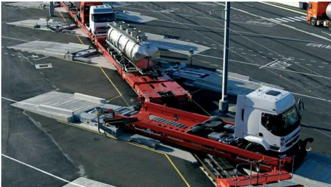
Figure 26. Loading station at the Modalohr terminal
