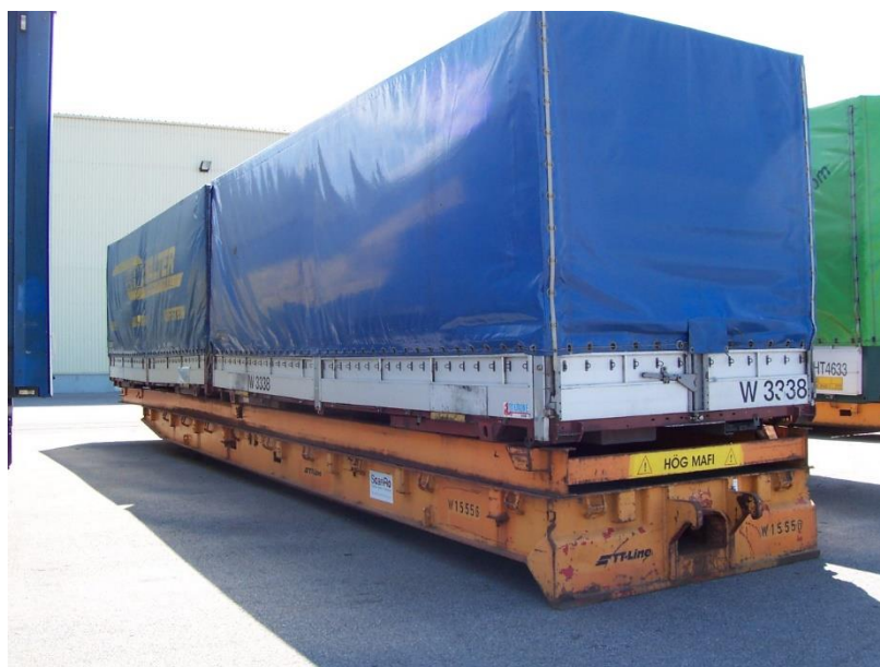
Figure 24. Roll trailer loaded with two swap bodies Source: photography by author of the analysis
